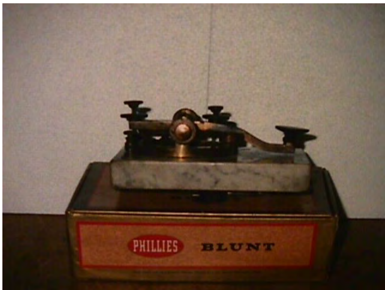
One of the Doron Brothers Electrical Co. marble-based “spark keys” (wireless telegraph). Saved for history by a private collector in Hamilton, Ohio
